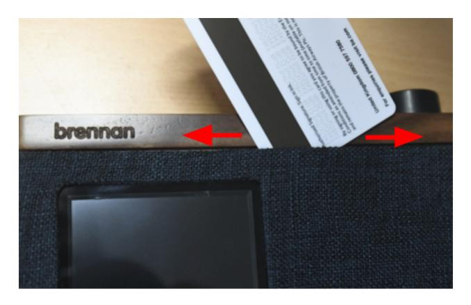
Step 6 - slide the cover off the body and replace SD.
