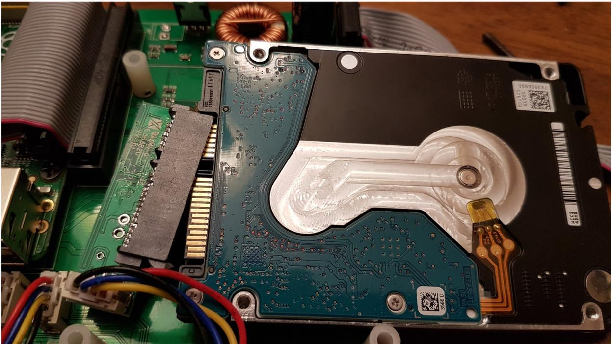
Don't pull on the cable. Just rock the little attached board side to side and it will come loose. I think mine had a small amount of glue on it originally. The glue just pulled off.
