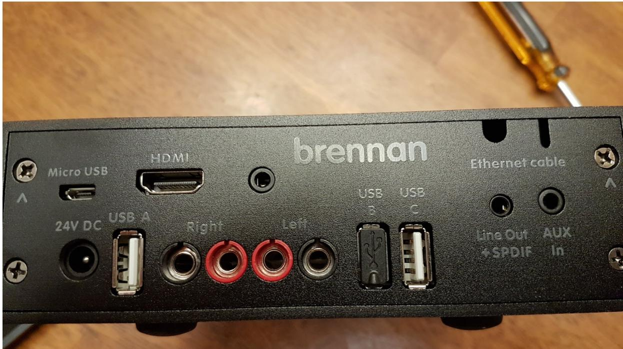
That will permit the whole internal assembly to be pulled out through the back. Pull it out about 4 inches (10cm) and stop!
