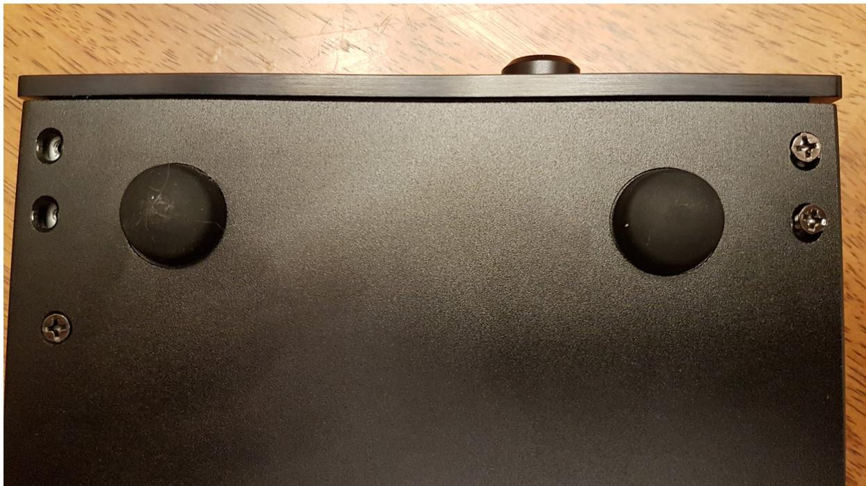
Once those 4 screws are removed the front panel can be pulled off (gently). You can remove the ribbon cable you see.
